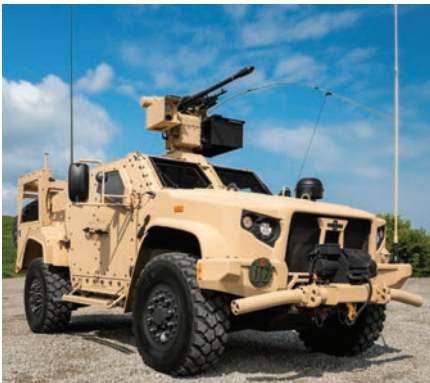
R400S Mk2 Dual with M230LF 30mm cannon and 7.62mm on the JLTV vehicle
