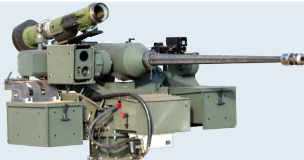
HEAVY GIMBAL: The R800S with MK44S 30x173mm and Javelin Missile
