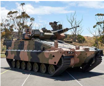
The T2000 with MK44S 30mm cannon and the R400S Mk2 D-HD with 12.7mm heavy machine gun on the Hanwha Defense Australia AS21 Redback vehicle
