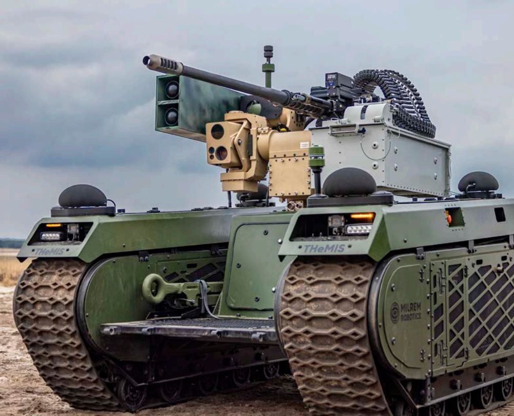
R400S on the Milrem Themis unmanned ground vehicle
