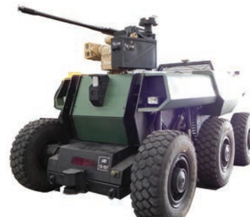
R400S with M230LF 30mm cannon on the IAI LR2 unmanned ground vehicle
