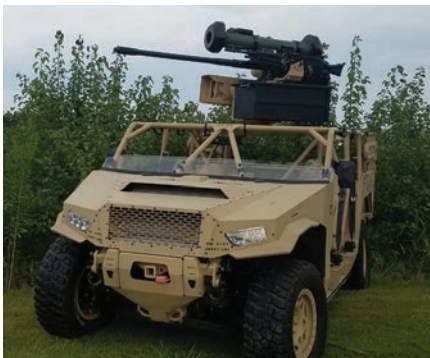
R400S Mk2-HD Dual with M230LF 30mm cannon, 7.62mm and Javelin missile on the Polaris Dagor vehicle
