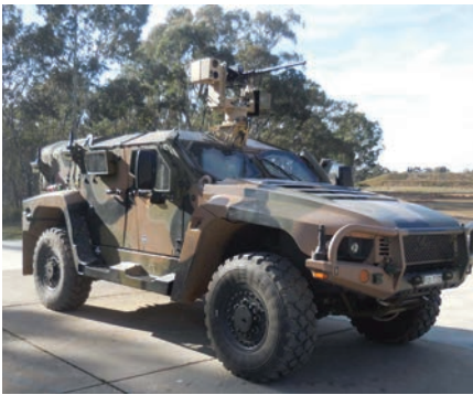
The R150S with 12.7mm heavy machine gun on the Hawkei vehicle
