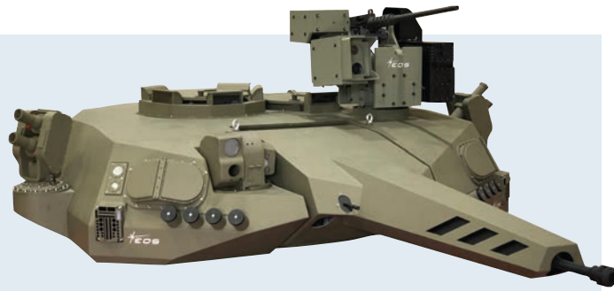
TURRET: The T2000 with MK44S 30x173mm cannon and R400S Mk2 D-HD with 12.7mm heavy machine gun
