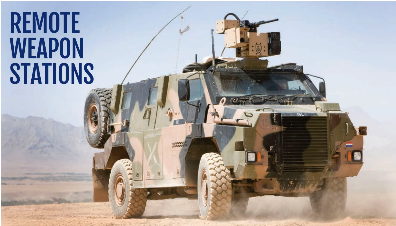
R400S Mk1 with 12.7mm heavy machine gun on the Dutch Bushmaster vehicle
